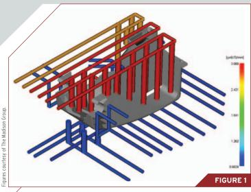
Simulation can help determine the flow rate required to achieve turbulent flow and minimize temperature rise.
