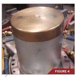
Image of mold with beryllium copper core cap.
