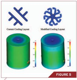
By modifying the current cooling layout the mold temperature within the core was reduced.
