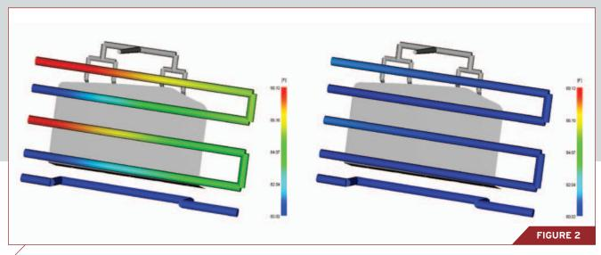
Ensuring turbulent flow minimizes the coolant temperature rise through the circuit.
