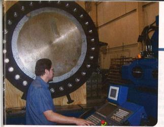
Carlson uses a specialized CNC cable gundrill deep-hole boring machine on a component of a heat exchanger for the oil and gas industry.
